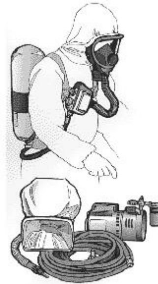
Air supplying respirators: Self-contained breathing apparatus (above) and line-supplied air respirator (pump placed in area for fresh (non-contaminated) air.
